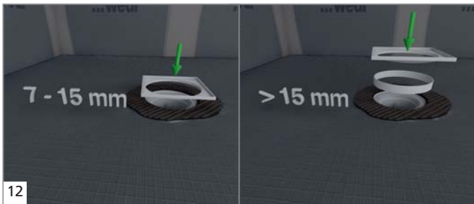
12 Bring the drain frame to the height of the top tile edge and secure in the bed of adhesive. If the tile is thicker than 15 mm, use the ramping element to adjust the height.
