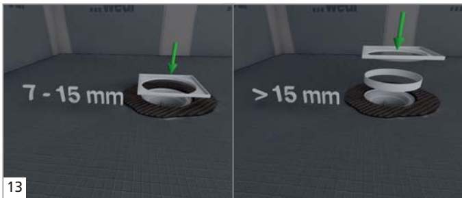
13 Bring the drain frame to the height of the top tile edge and secure in the bed of adhesive. If the tile is thicker than 15 mm, use the ramping element to adjust the height.
